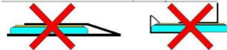
✓ **Solder Bridges** **焊接桥**
