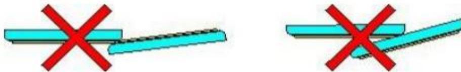
✓ *Batteries put in a Metallic Container or on a Metallic Plate 电池放在金属容器或金属板上*
